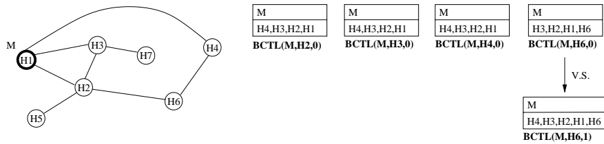
Fig. 10. Redundant forwarding prevention on stage 1.
