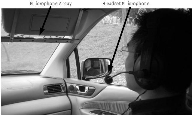
Fig. 3. Installation of the array inside the vehicle
