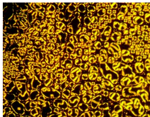
Figure 2. Polarizing optical micrograph of P1 : nematic droplet texture obtained at 150 °C.
