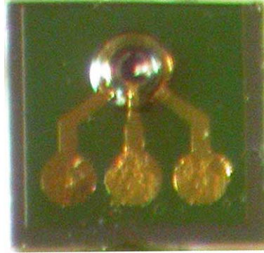
Fig. 2. Top-view photograph of the InGaAs MM-PINPD
