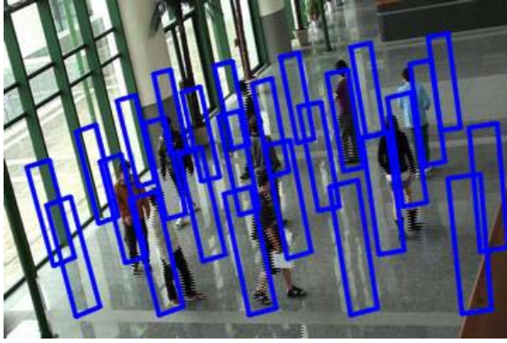
Fig. 3. Equally-spaced virtual billboards (VBs) of human size. The grid resolution is 160cm \times 160cm.
