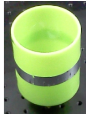
Fig. 6. (Color online) Prototype of cylinder with attached 1D diffuser.
