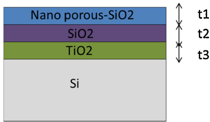
Fig. 2. Illustration of purely graded index ARC using planar multi-layer.
