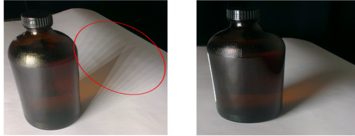
Fig. 13. (a) Multi-shadow effect of an anti-glare luminaire without the diffuser; (b) no multi-shadow effect with diffuser.
