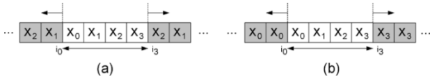
Fig. 6. Periodic symmetric and zero holding extension of signal. (a) Periodic symmetric extension signal; (b) Zero holding extension of signal.
