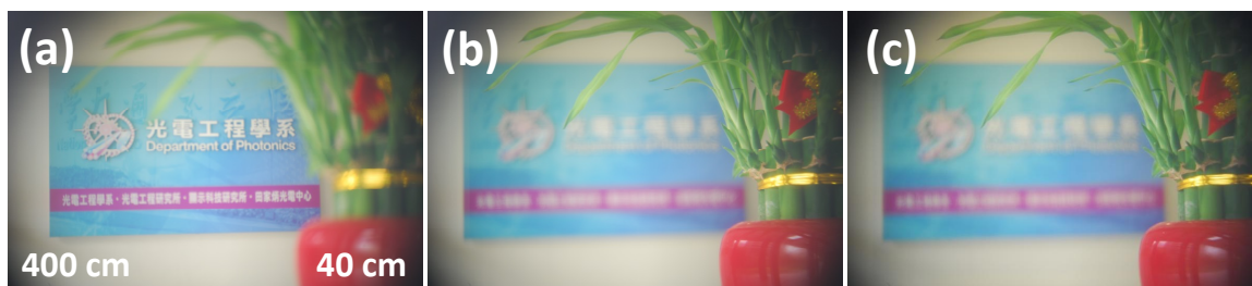
Fig. 4 The image performances of the polarized LC lens under ambient white light. (a) and (b) are operated in ES mode, while (a) and (c) are operated in ORW mode
