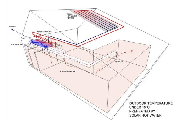
Figure 3.2.2.10 Heat Exchanger Preheated by Solar Hot Water Diagram
