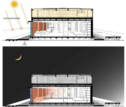
Figure 1.5.3 Thermal wall experiment diagram
