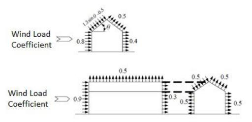
The lateral wind load applied on the structural system is smaller than that caused by earthquake. For the roof, it is also less than the live load. Therefore, it is not the controlling load case in the structural design.
