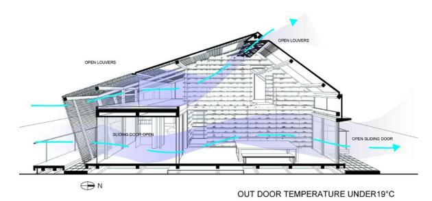
Figure 3.2.2.2 Natural Ventilation Diagram
