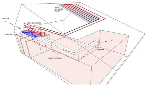
Figure 2.9.3 Solar hot water preheat air handling system
