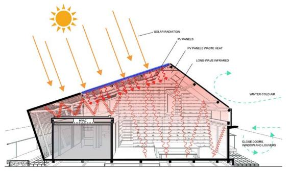
Figure 1.5.2 Greenhouse Effect Diagram
