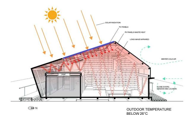
Figure 3.2.2.7 Greenhouse Effect Diagram
