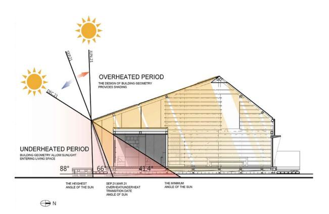
Figure 3.2.2.6 Solar Angle and Direct Solar Gain Diagram
