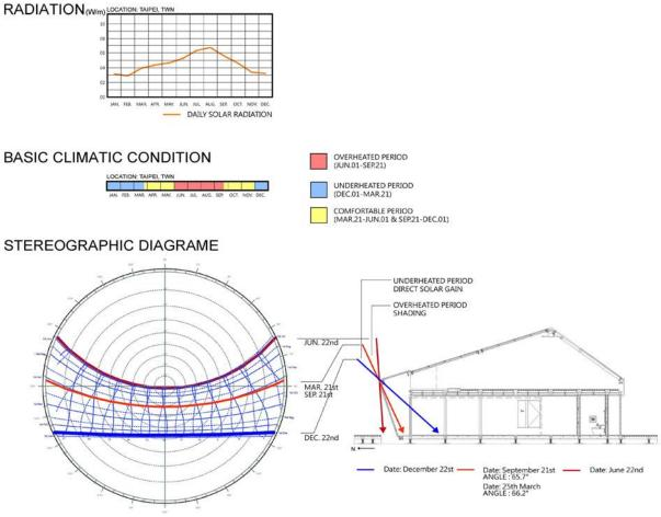
Figure 1.5.1 Solar Angle and Direct Solar Gain Diagram
