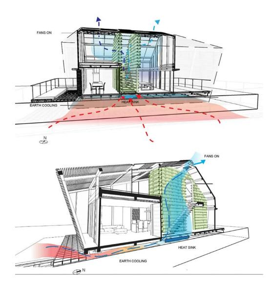
Figure 3.2.2.4 Earth and Vegetation Cooling Diagram
