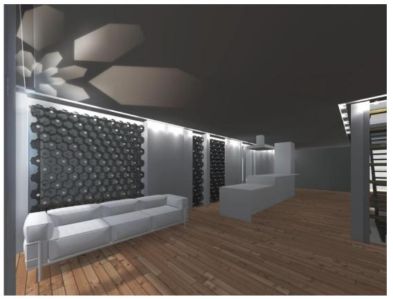
Fig.6.3.1 The lighting pattern on the ceiling The lighting pattern changes according to the electricity consumption in corresponding spaces.
