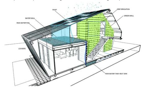
Figure 7.6.1 Rain water recycling system Diagram
