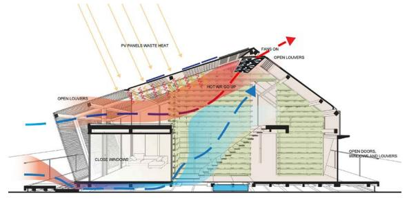
Figure 1.6.3 Solar Chimney Diagram
