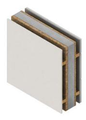
Figure 2.7.1 Glass Foam Insulation
