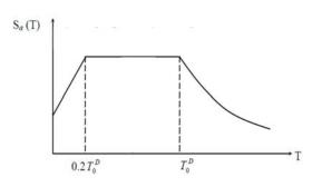
Figure 1.2.1 Earthquake Load in Taiwan
