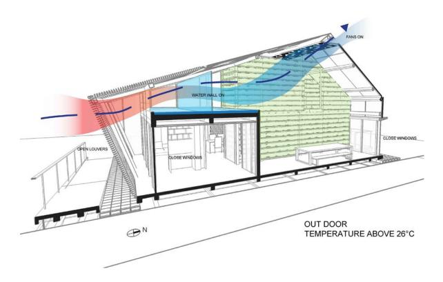
Figure 3.2.2.5 Evaporative Cooling Diagram
