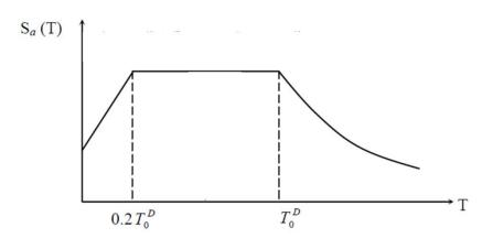
In this report, the structural period for the building located in Hsinchu is 0.358sec and the  $T_0^D$  is 0.7sec. Based on the Taiwan Seismic Design Specifications and Commentary of Buildings, the lateral load by earthquake will be
