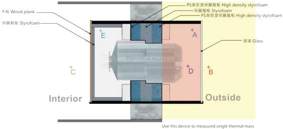
Use this device to measured single thermal mass unit temperature change in 3days and the relationship between indoor and outdoor temperature changes.
