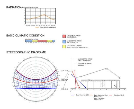
Figure 3.2.2.1 Solar Angle and Shading Diagram
