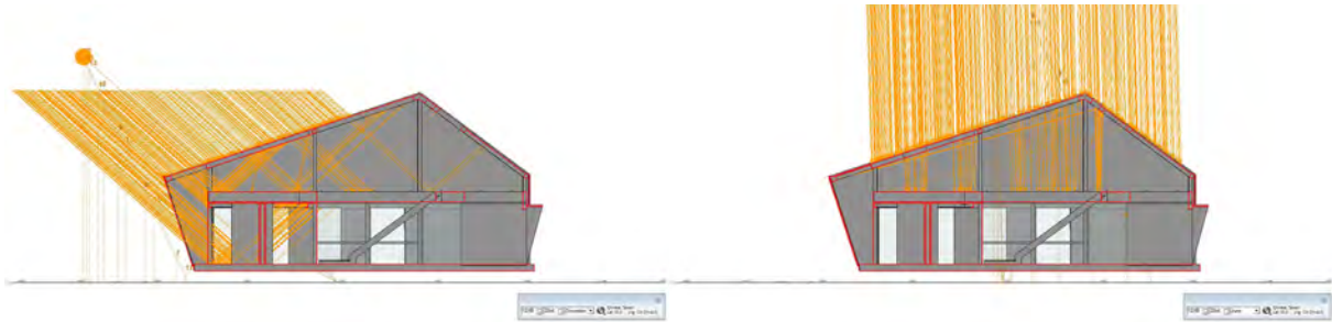
Figure 5.4.2.1.2a Solar exposure on building envelope during Winter Solstice
