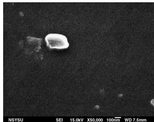
Fig. 6. The SEM top view of poly-Ge deposited on \text{SiO}_2 at 350^\circ\text{C} using conventional method.
