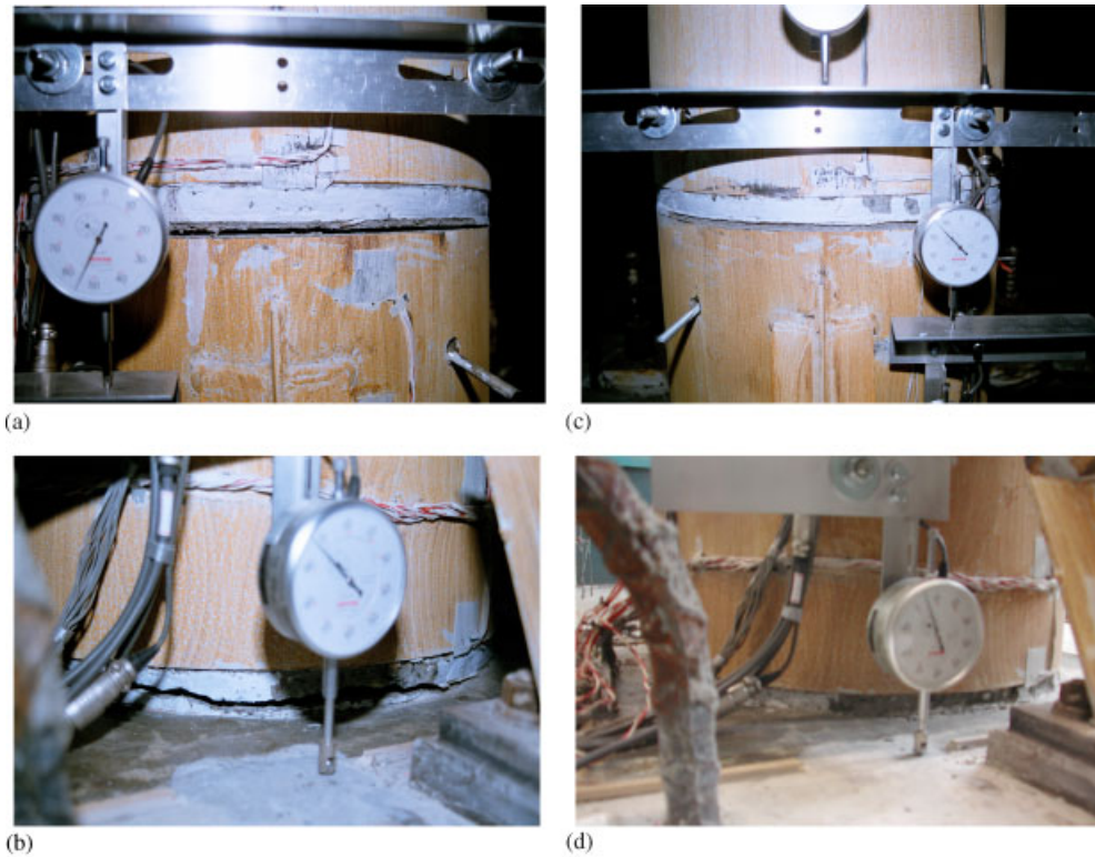
Figure 7. Specimen 2 at 4% drift: (a) opening between segments 1 and 2; (b) opening at base; (c) spalling between segments 1 and 2; and (d) crushing at base.
