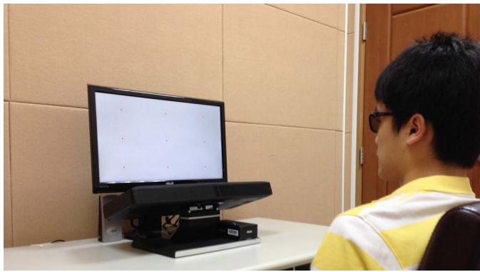
Figure 2. Experimental setup: 3D images are displayed on a 23-in. 3D display, and the Tobii TX300 eye tracker is used to track the user’s eye movement at a 120-Hz sampling rate.
