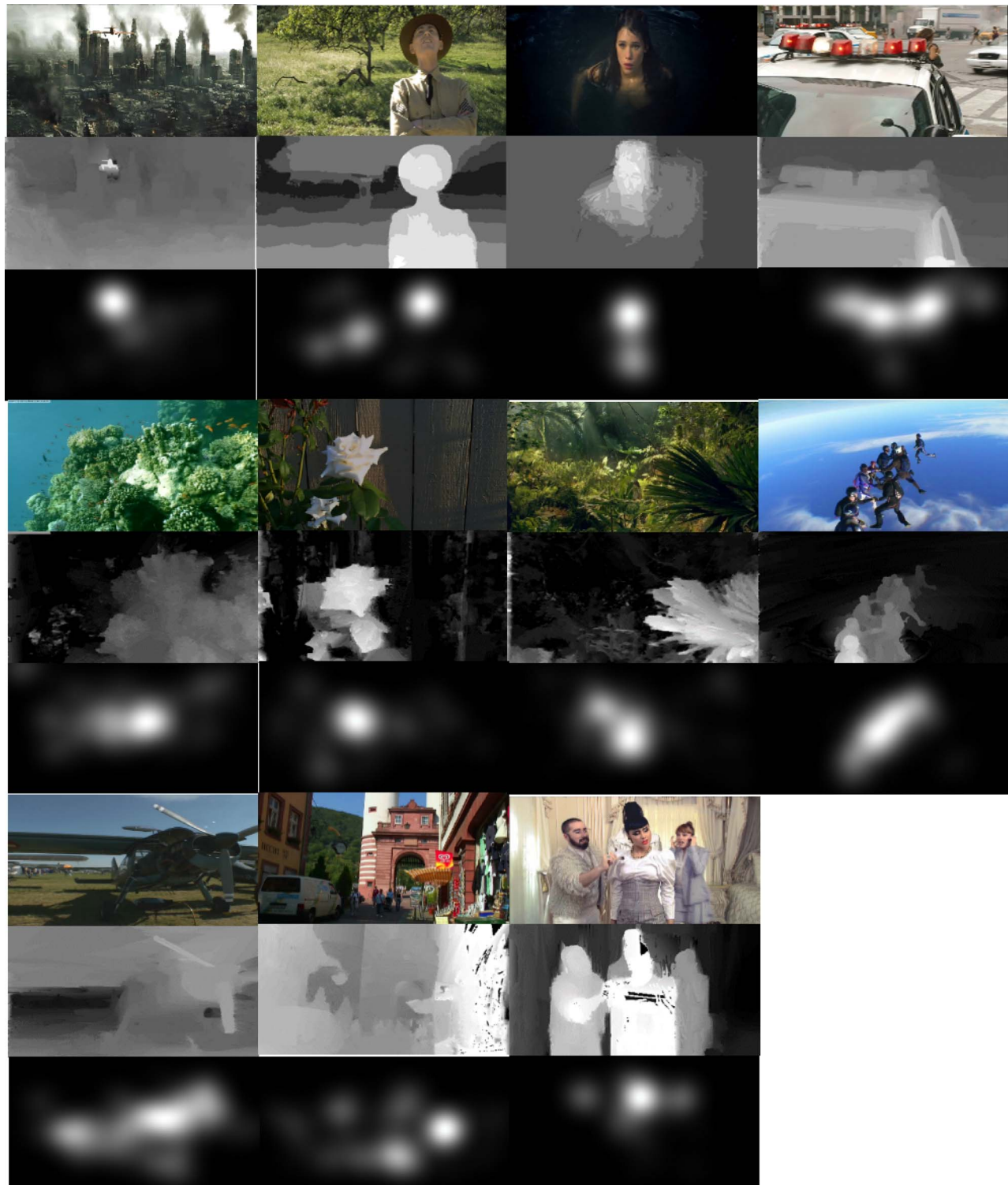
Figure 1. The 475 3D images captured from 11 3D videos, which come from YouTube and 3dtv. The depth maps are generated by DERS. The figure shows the original images (first row), the generated depth maps (second row), and the human fixation density maps (third row) in the NCTU-3DFixation database.
