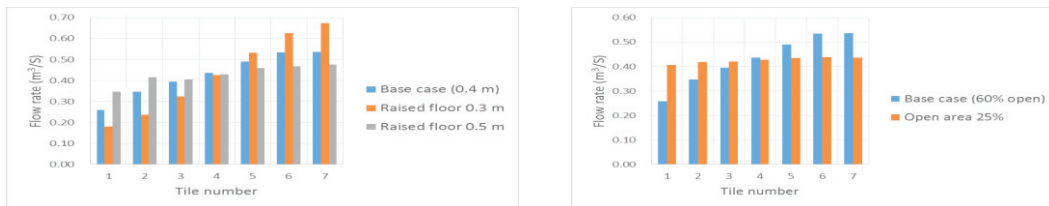
Fig. 4. (a) Effect of the height of raised floor; (b) Flow rate for 60% open area and 25% open area
