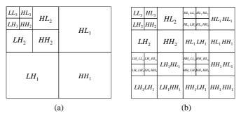
Fig. 3. The wavelet transform applied to C(x, y) in the case of three embedded images.
