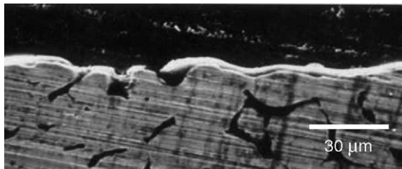
Fig. 8. The cross-section view of PASS specimen after mechanical grinding with 200-grit emery paper.
