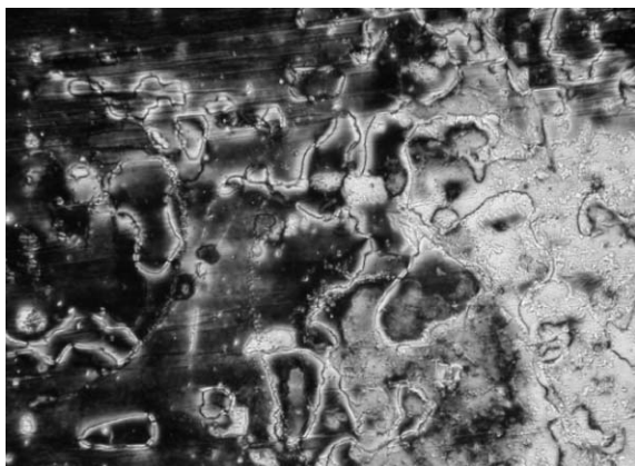
Fig. 1 A micrograph showing the contact preparation of 1c (right) with 3-cyano-8-hexyloxy-biphenylene (left) at 50 °C on cooling.
