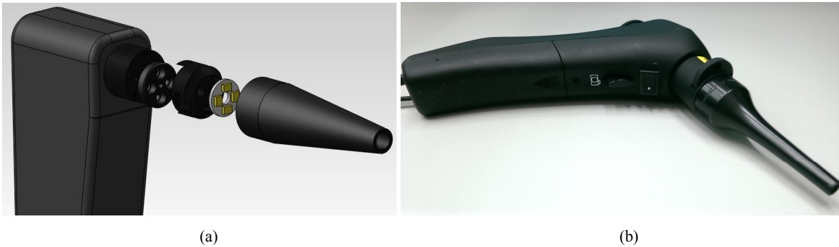
Figure 2. (a) The construction drawing of the portable LIAF imager; (b) the embodiment of the portable LED Induced Autofluorescence (LIAF) imager.
