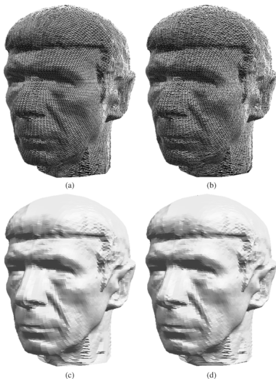
Fig. 8. Visualization of the transparency test: (a) original Spock model rendered in a wireframe format; (b) watermarked Spock model rendered in a wireframe format; (c) original Spock model rendered in a flat-shaded form; and (d) watermarked Spock model rendered in a flat-shaded form.
