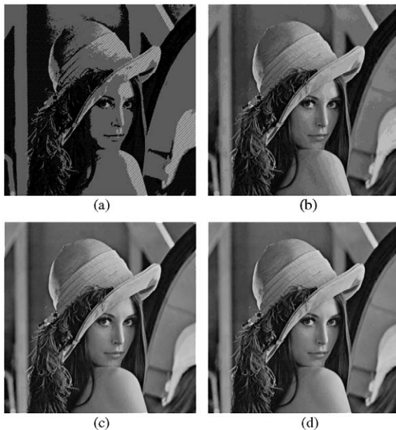
Fig. 5. The recovered images revealed from various numbers of stego images: (a) from any 2 stego images ( PSNR = 14.57); (b) from any 3 stego images ( PSNR = 29.28); (c) from any 4 stego images ( PSNR = 48.46); (d) from any 5 stego images (lossless).
