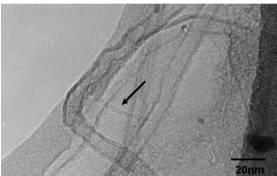
Fig. 2. Typical HRTEM micrographs of the synthesized CNTs using AlON buffer layer material.
