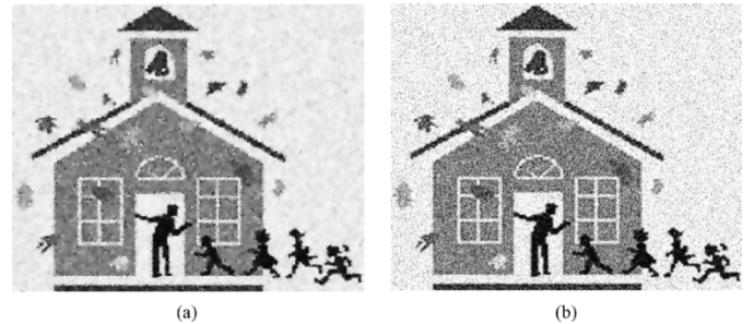
Fig. 11. (a) Original image and (b) grayscale image captured by the test chip under V_{com} of 1.79 V.
