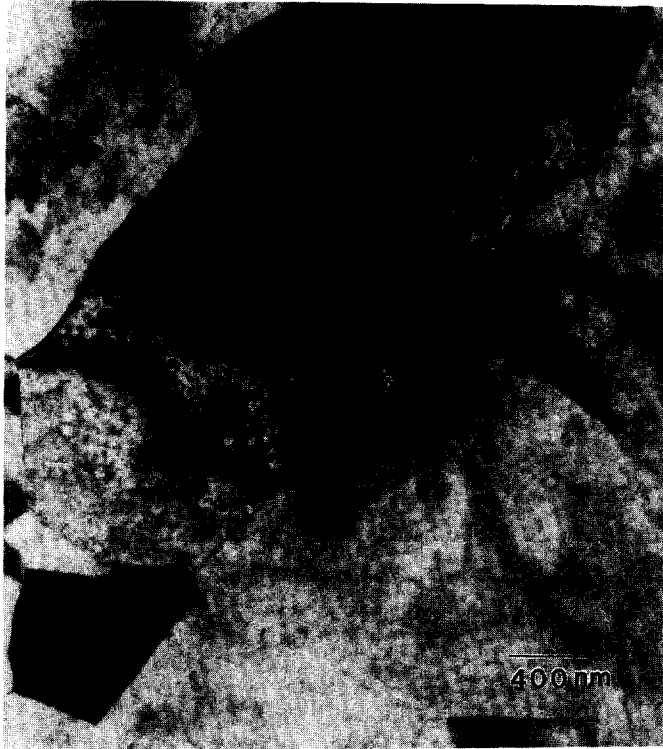
Figure 1. Planar TEM image shows a twinned silicon precipitate at aluminum grain boundary (A).
