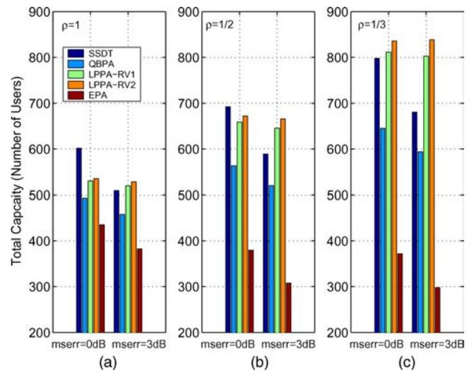
Figure 13. Total capacity performance with and without measurement error for EPA, QBPA, SSDT, LPPA-RV1 and LPPA-RV2 techniques in the (a) homogeneous cellular system, (b) heterogeneous cellular system with  $\rho = 1/2$ , (c) heterogeneous cellular system with  $\rho = 1/3$ .
