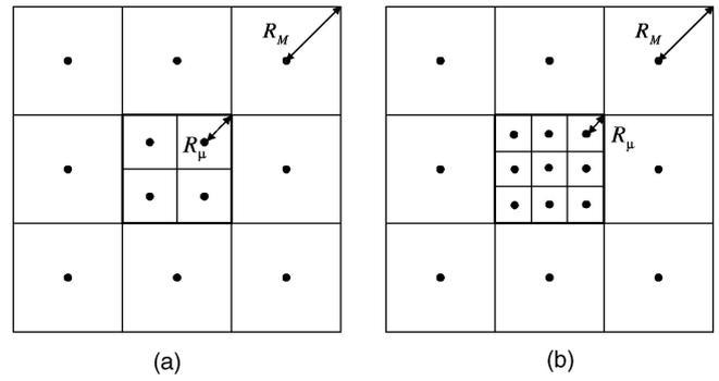
Figure 6. Examples of heterogeneous cellular network (a)  $\rho = 1/2$ , (b)  $\rho = 1/3$ .
