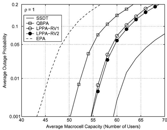
Figure 7. Averaged outage performance in the homogeneous cellular systems ( $\rho = 1.0$ ) for the EPA, QBPA, SSDD, LPPA-RV1 and LPPA-RV2 techniques.
