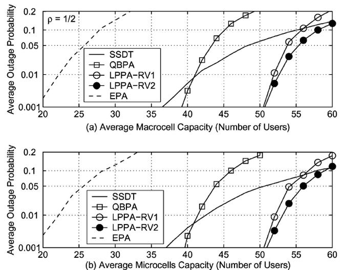
Figure 10. Averaged outage performance in the heterogeneous cellular systems ( $\rho = 1/2$ ) subject to measurement errors for EPA, QBPA, SSDD, LPPA-RV1 and LPPA-RV2 techniques.
