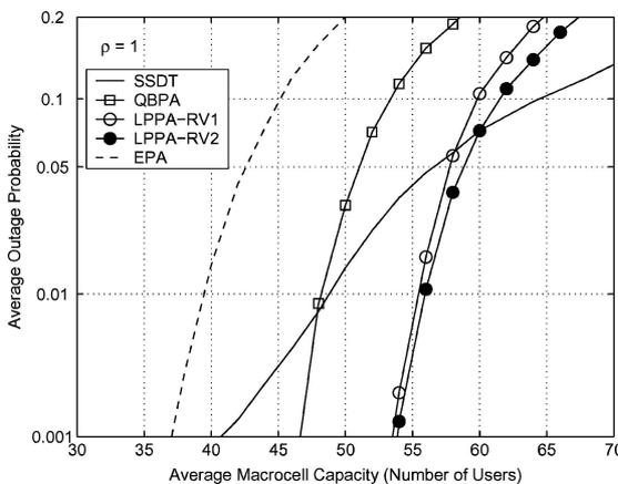
Figure 8. Averaged outage performance in the homogeneous cellular systems ( $\rho = 1.0$ ) with measurement error for the EPA, QBPA, SSDD, LPPA-RV1 and LPPA-RV2 techniques.
