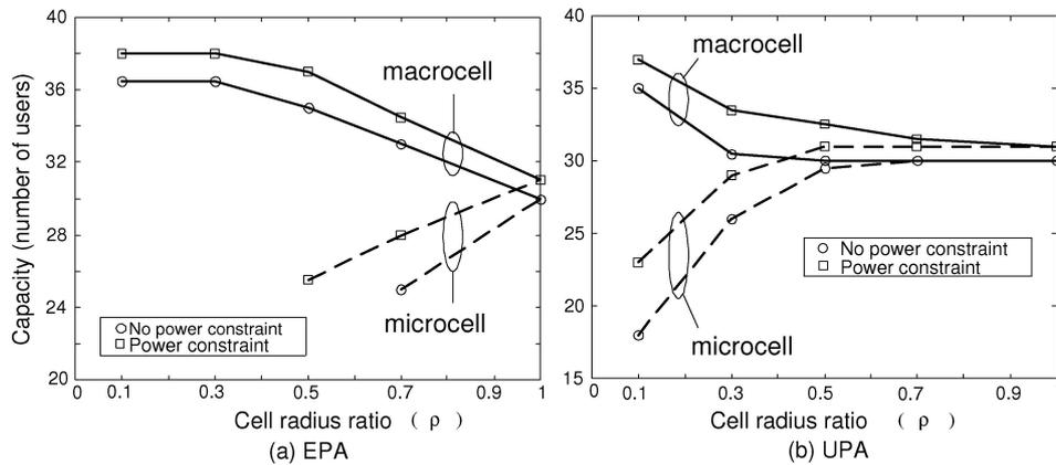
Figure 4. Capacity of (a) equal power allocation (EPA) and (b) unequal power allocation (UPA) with soft handoff against the ratio of radius of the microcell to that of the macrocell  $\rho$ .
