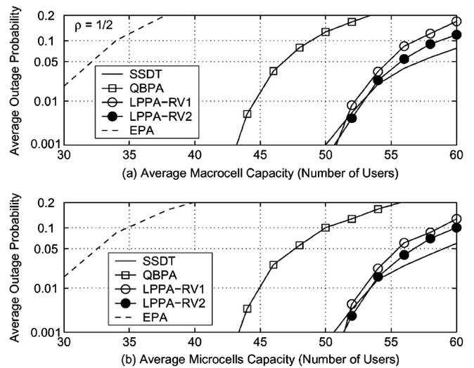
Figure 9. Averaged outage performance in the heterogeneous cellular systems ( $\rho = 1/2$ ) for the EPA, QBPA, SSDD, LPPA-RV1 and LPPA-RV2 techniques.
