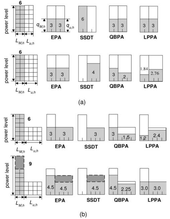
Figure 3. Example for different soft handoff downlink power allocation techniques. (a) homogeneous cellular system and (b) heterogeneous cellular system.
