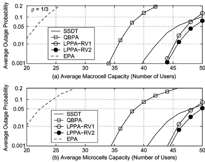
Figure 11. Averaged outage performance in the heterogeneous cellular systems ( $\rho = 1/3$ ) for the EPA, QBPA, SSDT, LPPA-RV1 and LPPA-RV2 techniques.
