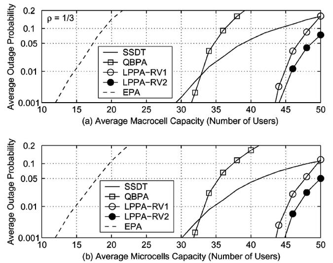
Figure 12. Averaged outage performance in the heterogeneous cellular systems ( $\rho = 1/3$ ) subject to measurement errors for the EPA, QBPA, SSDT, LPPA-RV1 and LPPA-RV2 techniques.
