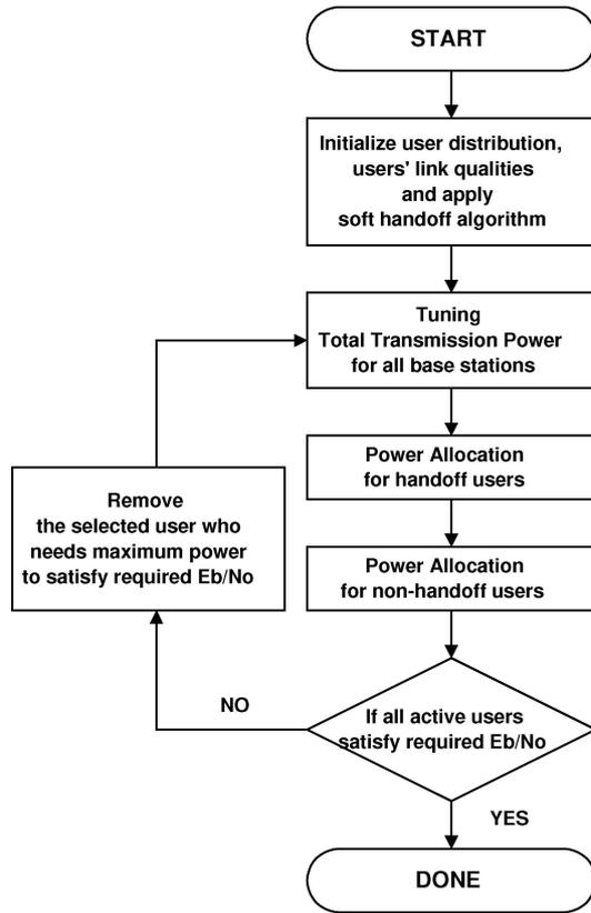
Figure 5. Flowchart of a generic joint resource allocation mechanism integrating four key techniques: (1) soft handoff, (2) downlink power allocation for handoff users, (3) downlink power control for non-handoff users, and (4) removal procedures.
