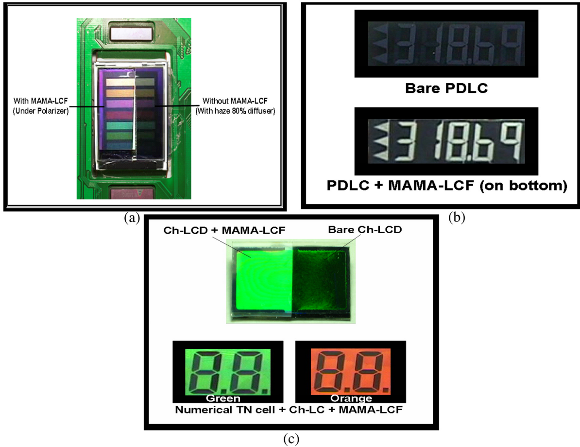
Fig. 17. Sample photographs of: (a) color-STN LCD, (b) PDLC, and (c) Ch-LCD. The displays with MAMA-LCF clearly show much better image quality. (Color version available online at http://ieeexplore.ieee.org .)
