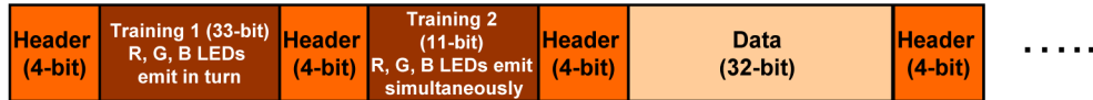
Fig. 3. Structure of the data packet, including the training signal 1 and 2 for MIMO; and each packet is consisted of a header and payload.
