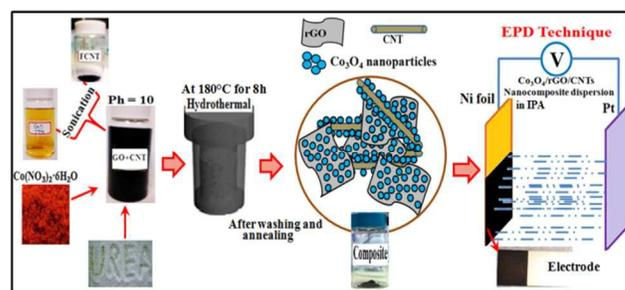
Fig. 1. Scheme of Co<sub>3</sub>O<sub>4</sub>/rGO/CNT nanocomposite synthesis and the process of electrodes fabrication.
