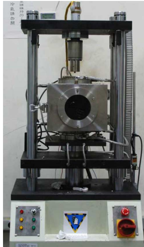
Fig. 1. Ultrasonic hot upsetting experiment set up.
