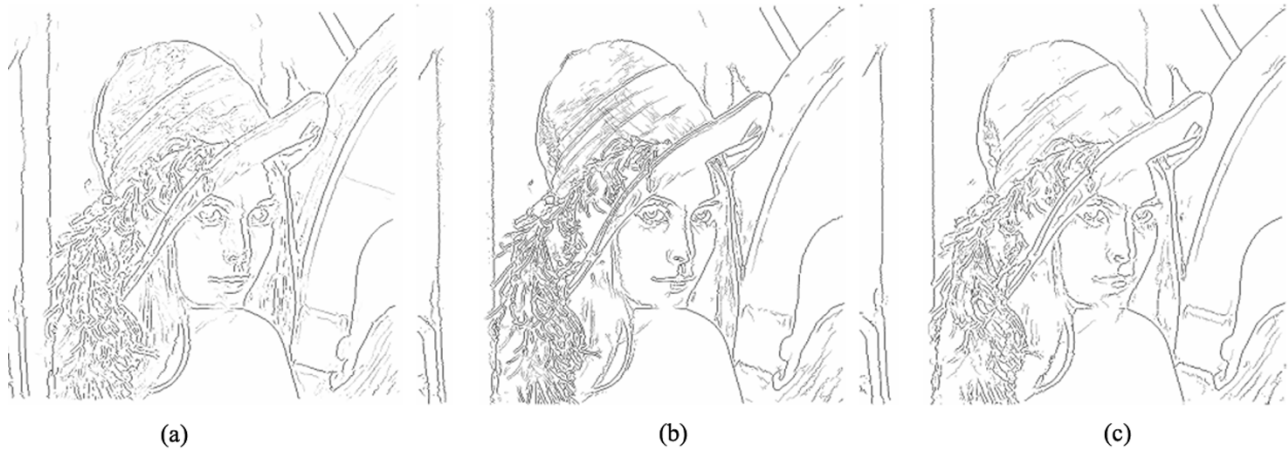
Fig. 14. (a) Edge detection based on verge points. (b) Edge detection based on the Canny Operator, where \sigma_m is set as 1 and the low- and high-hysteresis thresholds are set as 0.0375 and 0.0938, respectively. (c) Edge detection based on the Canny Operator, where \sigma_m is set as 2 and the low- and high-hysteresis thresholds are set as 0.0375 and 0.0938, respectively. The gray-level value represents the edge strength. The averaged edge strengths of these three figures are adjusted to be equal.
