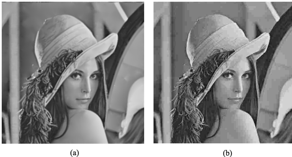
Fig. 13. Illustrations of two different compression algorithms. (a) Reconstructed image using the proposed method; compression rate = 31.12, PSNR = 28.67. (b) Reconstructed image using JPEG compression, compression rate = 31.08, PSNR = 30.65.
