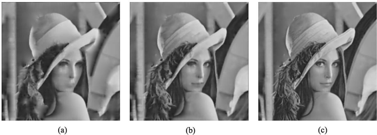
Fig. 11. Progressive image reconstruction. (a) Using “top-layer” verge curves only; totally, 8219 verge points. (b) Using “top-layer” and “middle-layer” verge curves; totally, 11 523 verge points. (c) Using all verge curves; totally, 15 926 verge points.
