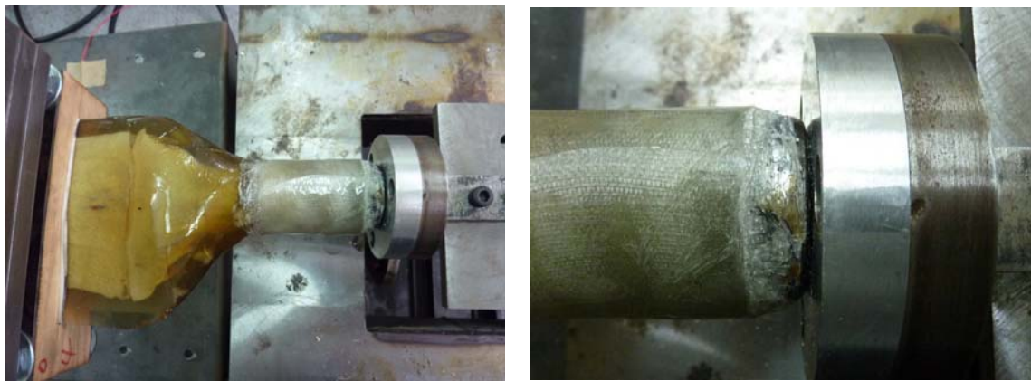
Figure 12: SCWTBs in root repair
