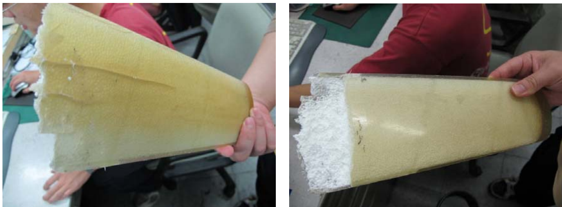
Figure 13: Blade destruction (1) Leeward & (2) Windward
