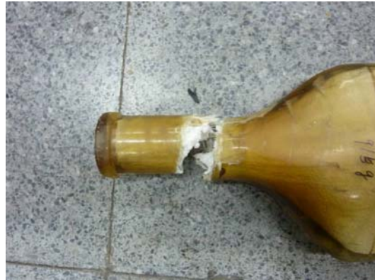
Figure 11: Destruction of root and metal joints
