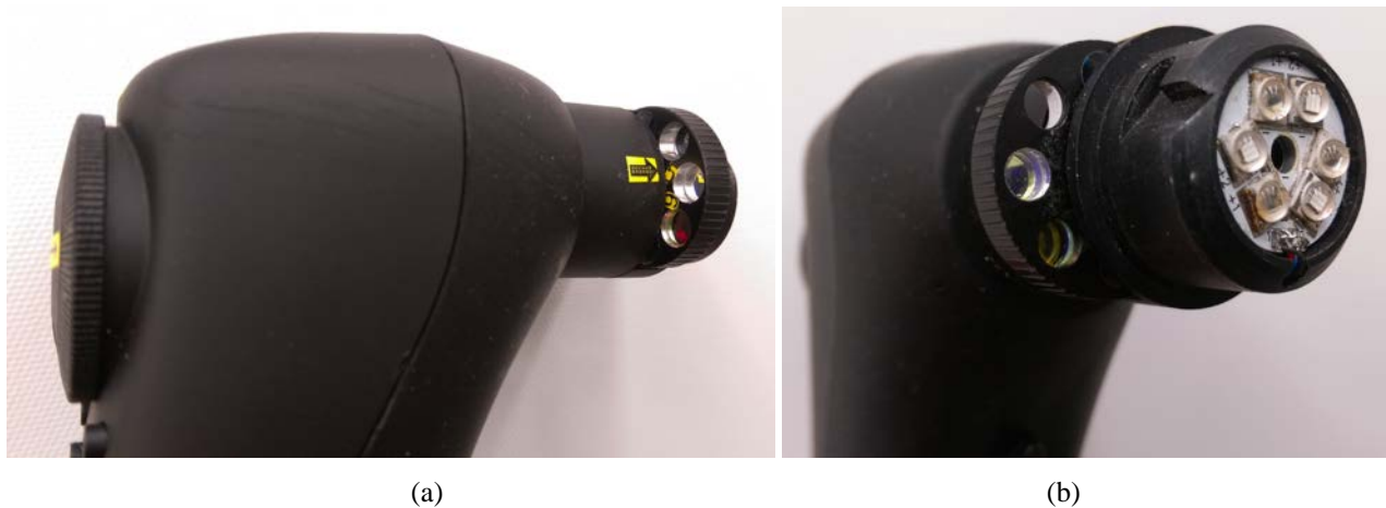
Fig. 3. (a) The side view and (b) the front view of the rotary filter ring contains eight holes for holding the filters
