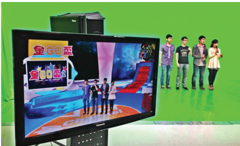
Figure 1. Virtual studio removes a range of green or blue color from the image captured by a studio camera and replaces it with a 3D virtual environment 1
