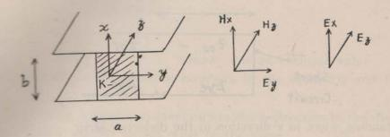
$\mathbb{E}_z$ ,  $H_x$  and  $H_z$  are normally required for parallel-plate waveguide. The two additional components  $E_x$  and  $E_z$  are necessary to satisfy the boundary conditions at the air-dielectric interface.
