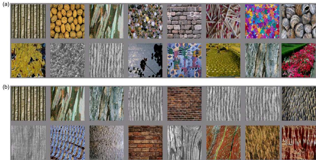
Fig. 7. An example of texture retrieval given a directional texture as query image using MPEG-7 HTD. (a) Retrieved result without prescreening. (b) Retrieved result with prescreening.
