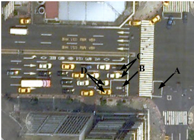
Fig. 4. A top-view of the experimental intersection with four waiting areas marked (taken from Google Map).
