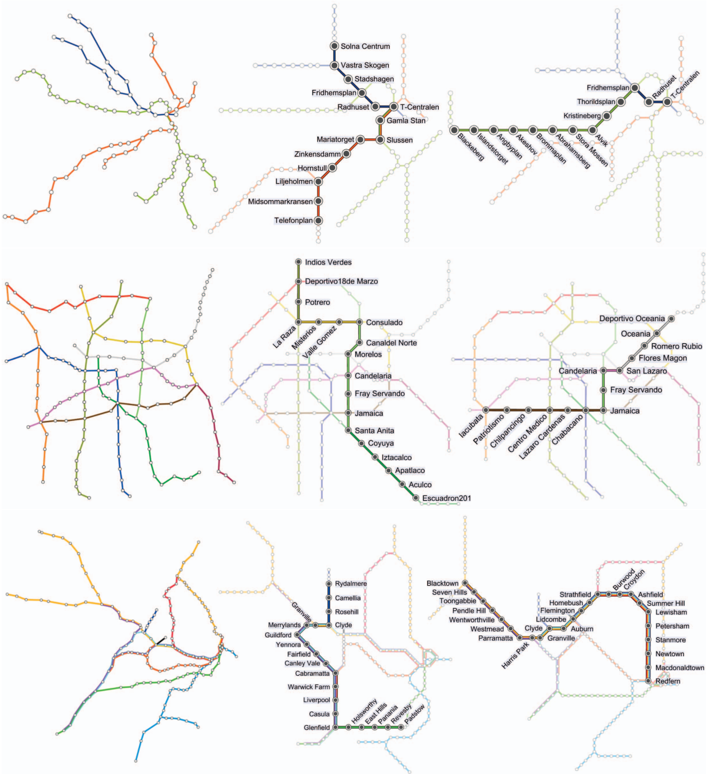
Fig. 9. From top to bottom are the metro maps of Stockholm, Mexico City and Sydney. (left) The geographic layouts. (middle and right) The focus+context results are automatically determined using our system.
