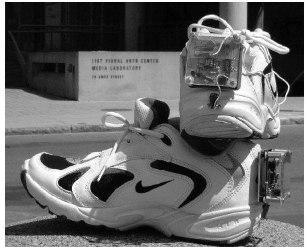
Fig. 22. Piezoelectric-powered RFID shoes with mounted electronics by Shenck and Paradiso in 2001 [20].
