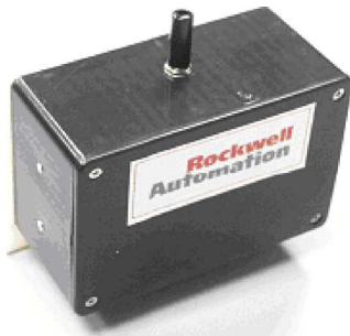
Fig. 30. A self-powered sensor node by Discenzo et al. in 2006 [97].
