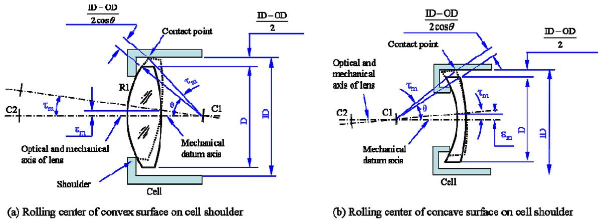
Fig. 4 Rolling center of optical surface on cell shoulder
