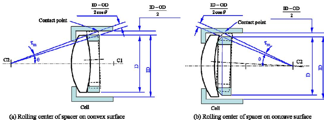
Fig. 5 Rolling center of spacer on lens surface
