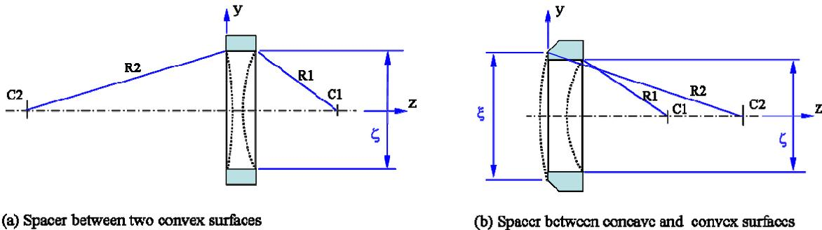
Fig. 8 Tolerance model of spacers
