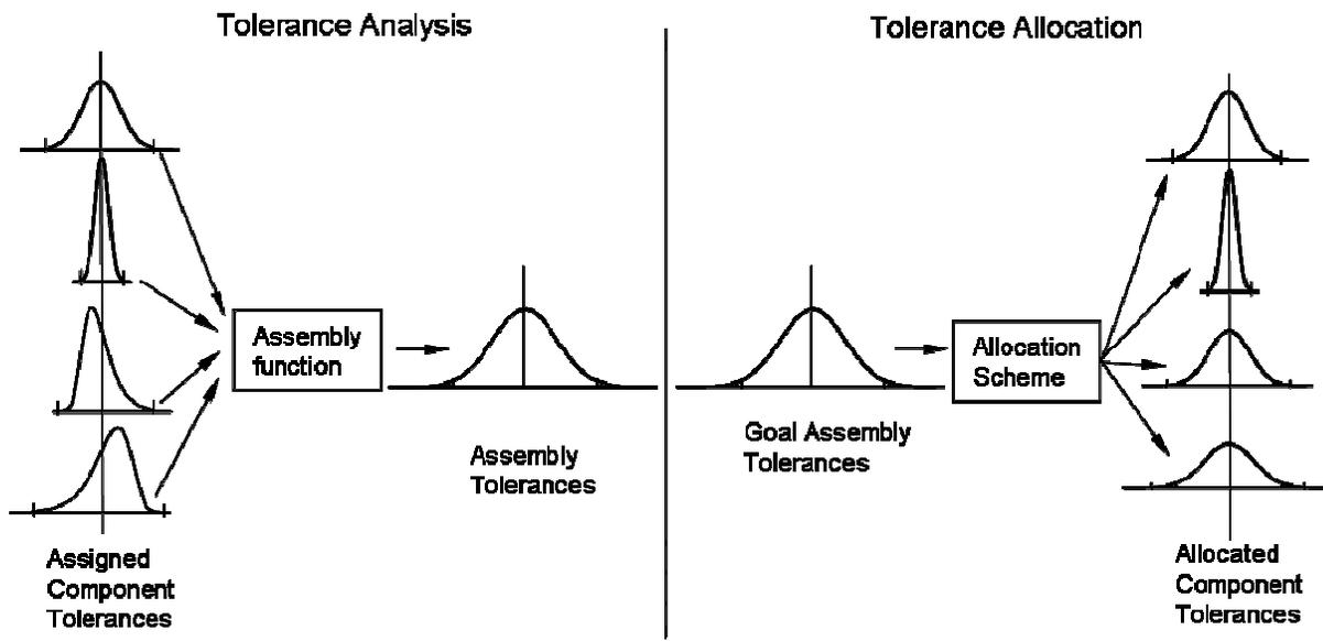
Fig.1 Comparison of tolerance analysis and tolerance allocation
