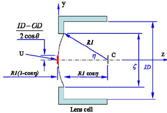
Fig. 7 Tolerance model of cell
