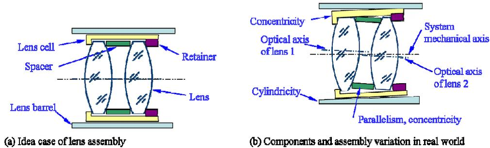
Fig. 2 Lens mounted in barrel
