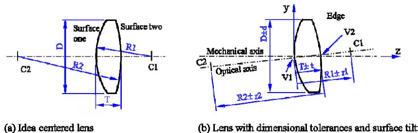
Fig. 3 Tolerance model of a convex lens
