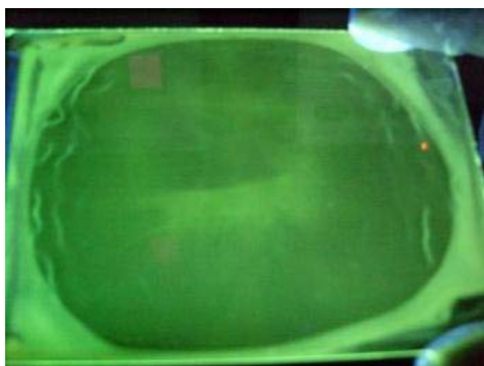
FIG. 4. (Color online) The image of the organic layers. The first organic layer is dissolved and the square is disappeared when much solution is used to form the second organic layer.
