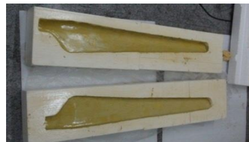
Figure 2. Mould for blade fabrication.
