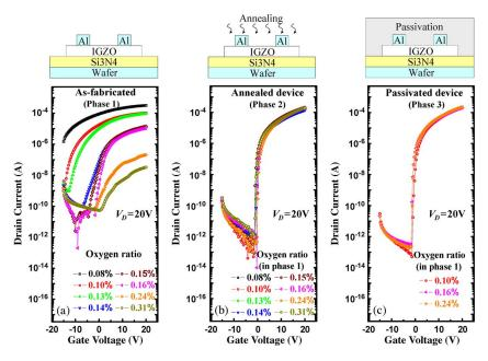
Fig. 1. Transfer characteristics of (a) as-fabricated, (b) annealed, and (c) passivated devices fabricated under various oxygen ratios during active layer deposition.
