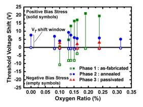
Fig. 2. Threshold voltage shifts after examinations of both positive and negative bias stresses, with each stress applied for 5000 s, plotted as a function of the oxygen ratio used during IGZO layer deposition. The devices in three fabrication phases were compared: as-fabricated, annealed, and passivated devices.
