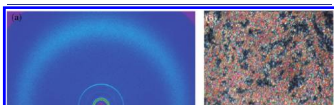
Figure 2. (a) GIWAXS pattern and (b) POM image of the surface-aligned sample of the covalent-bonded compound C–SiO at 100^\circ\text{C} .
