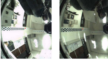
Fig. 17. Picked-out pairs of corresponding pixels in two omni-images (marked by two red dots).
