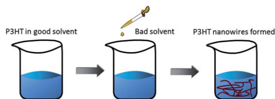
Fig. 9 Schematic illustration of using the mixed-solvent method to make P3HT nanowires. The P3HT polymers are first dissolved in a good solvent. After the bad solvent is added, P3HT polymers start to aggregate and P3HT nanowires are formed.
