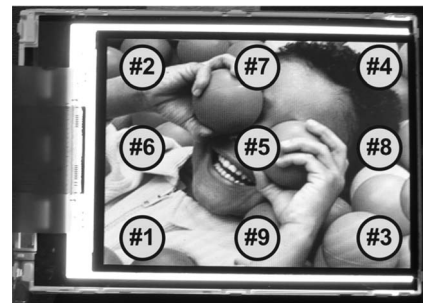
Fig. 12. Test point definition on display panel under system-level ESD tests with air-discharge test mode.
