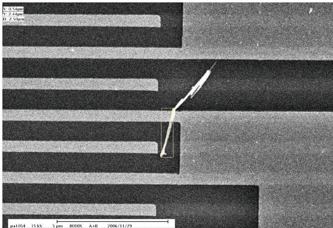
Figure 2. SEM image of a single \text{Sb}_2\text{Se}_3 nanorod on the patterned substrate.
