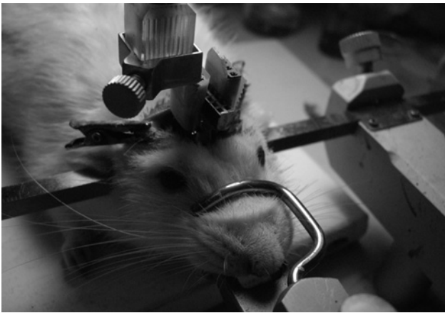
Fig. 2 Placement of an EEG electrodes and cooler modules in a head of rat
