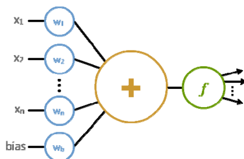
Fig. 1. One of the neurons of the input layer in a neural network, where x_1 to x_n are the n inputs, w_1 to w_n are the weights for the inputs, w_b is the bias, + stands for summation, and f is the activation function.
